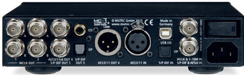
ABOVE: Socketry accommodates dual Word clock(s), AES3 and S/PDIF digital ins and outs on BNC, S/PDIF outs on RCA coax and Toslink optical, balanced AES/EBU in and out on XLR plus the addition to this latest MC-3 model – a USB 2.0 interface
