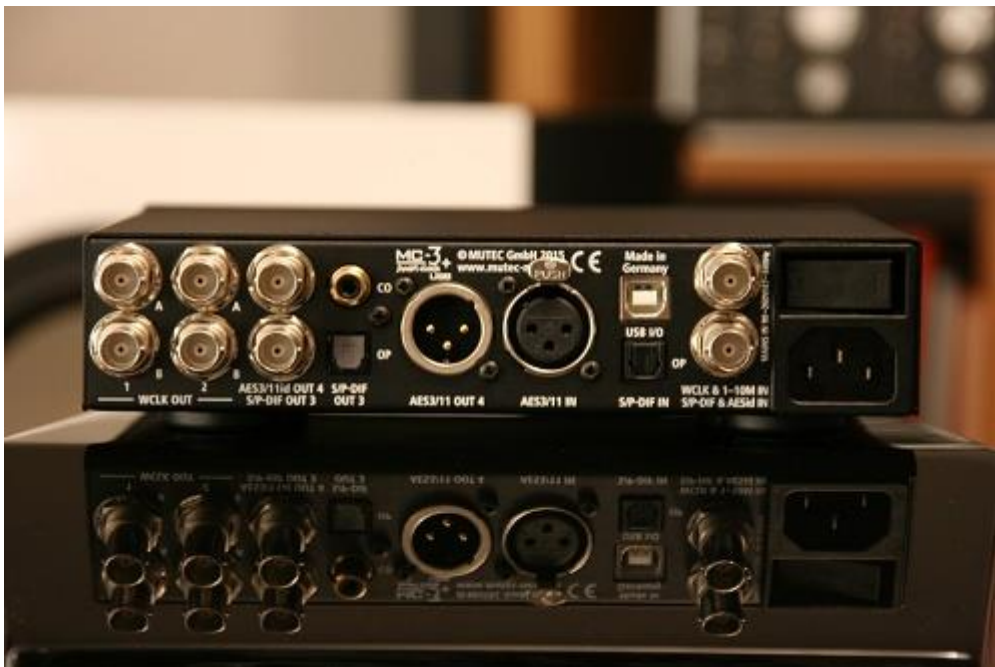
Picture 2: The rear panel has been filled to last fraction of an inch and is fully loaded. Coax S/P-DIF input is only possible via BNC (bottom right), which may require an additional RCA-to-BNC adapter depending on the available cable.
